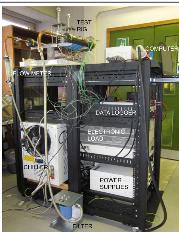
Fig. 1. The complete measurement system used for the experiments.
